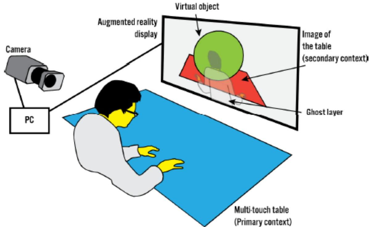
Fig. 1. Setup of Multi-touch augmented reality system
