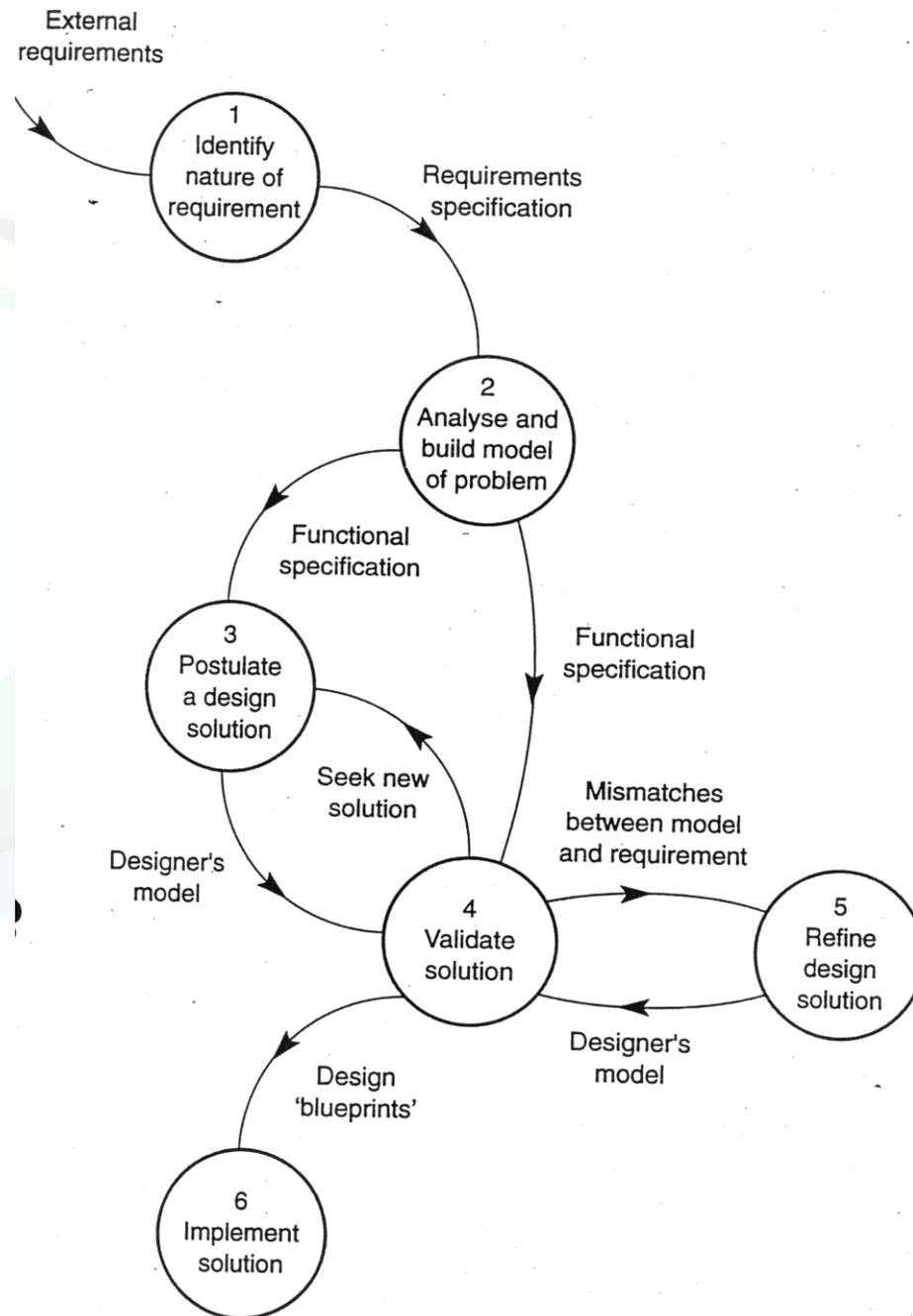
Figure 1.2 A model of the design process.
