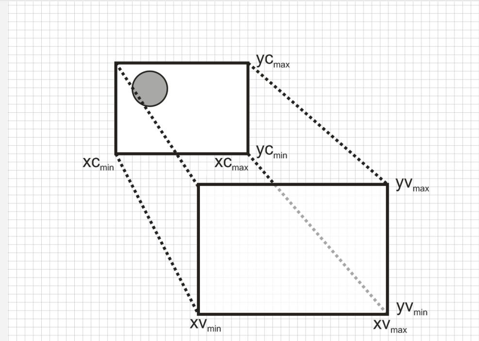
$$(x_v, y_v, 1) = (x_p, y_p, 1) \begin{pmatrix} s_x & 0 & 0 \\ 0 & s_y & 0 \\ -s_x xc_{\min} + xv_{\min} & -s_y yc_{\min} + yv_{\min} & 1 \end{pmatrix}$$
